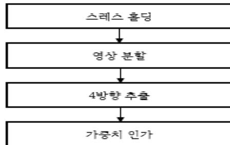
Fig. 4 Flowchart of edge detection
