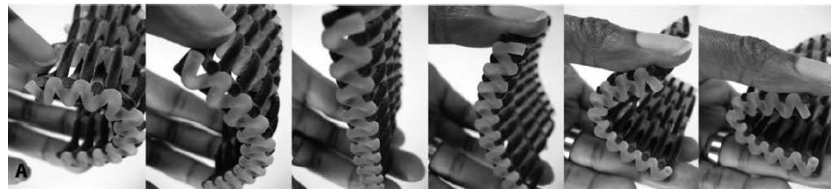
Figure 5. 3D Printed Weave with Rubber Warp and Black ABS Plastic (papers.cumincad.org)
