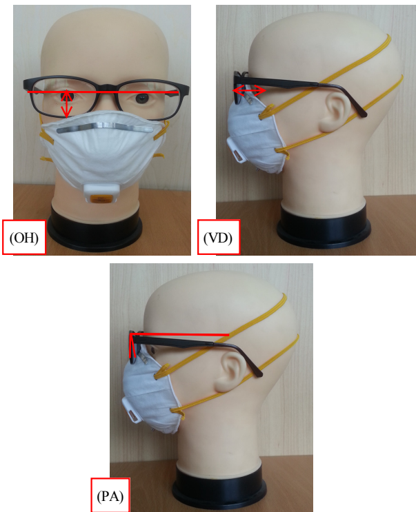
Fig. 2. Standard and change point of glasses fitting factors and donning state according to first choice.
