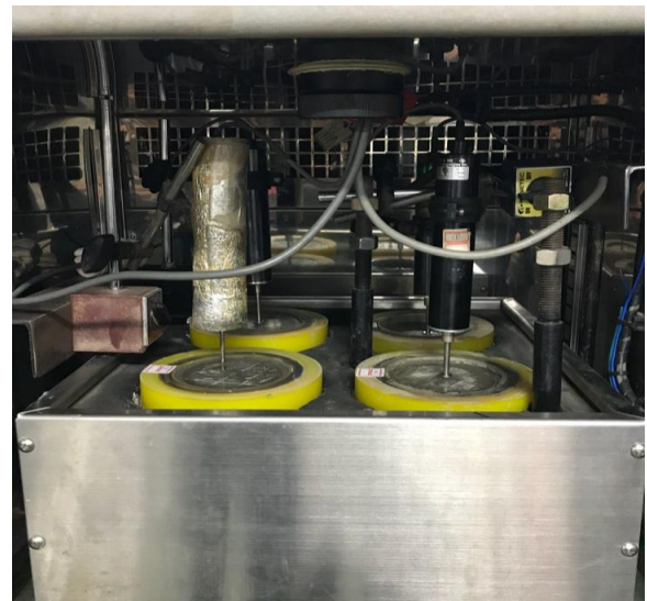
Fig. 6. Frost heaving test using temperature controller
