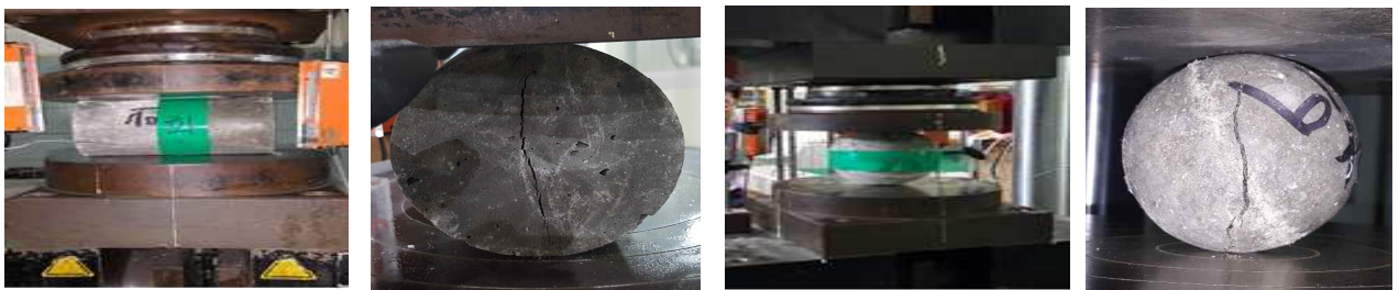
(a) Cylinder Specimen (b) Crack Propagation (c) Sphere Specimens (d) Crack Propagation Fig. 3. Split Test and Crack Propagation of Specimens
