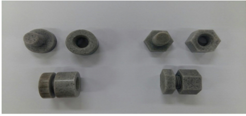
Fig. 9. The manufacture of the PMMA/Alumina composite sample containing 7 wt. % alumina.
