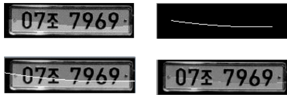
Fig. 7 Example of Curved Lines and Shadow Removal Images using the Least Squares Method
