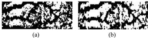
Fig. 5 The comparison of binarization result (a) The result of iterative threshold selection method (b) The result of P-tile binarization method
