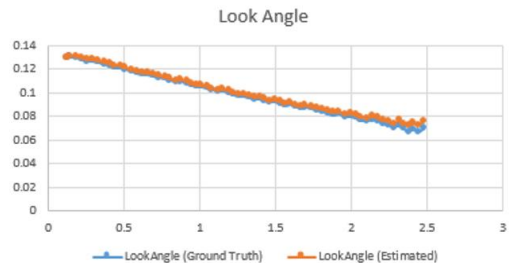
Fig. 15. Look angle(rad) vs time(sec) with Simulink
