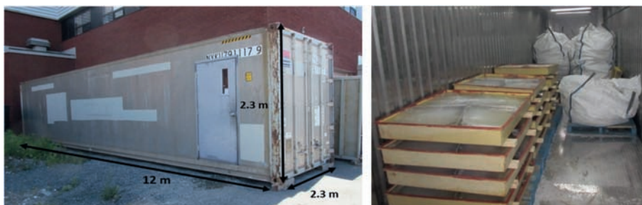
Fig. 4. Ice rubble production and storage inside the refrigerated container.
