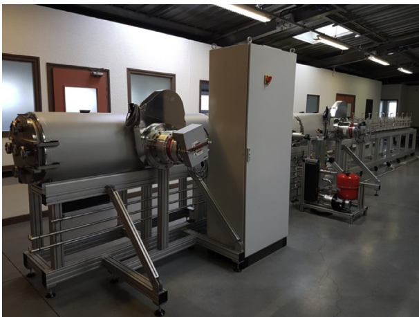
Fig. 3. Picture of the current status of fabrication of the full-length Cr coating deposition prototype.
