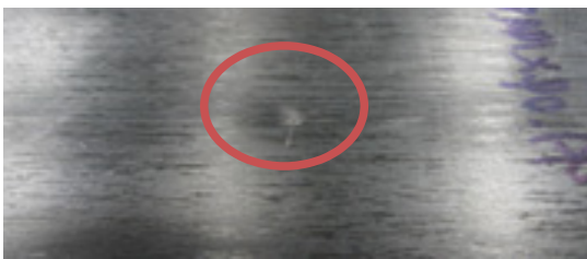
Fig. 7. Failure mode of the composite (dent/depression)
