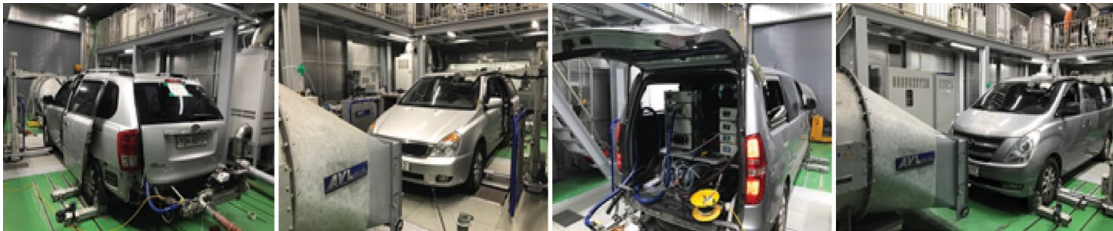
Fig. 5. Photographs of correlation test for PEMS vs CVS.
