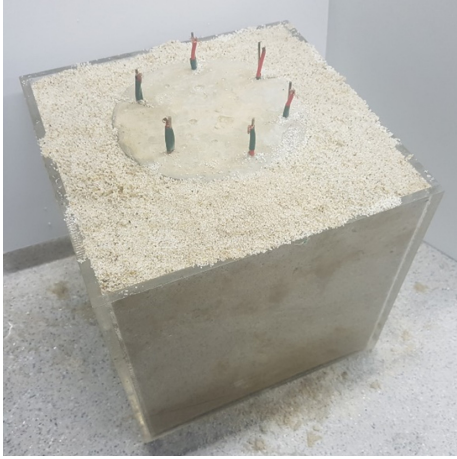
Fig. 5. Small-scale model pile embedded in soil
