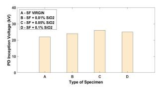
Fig. 2. Partial Discharge Inception Voltage values for virgin and nano modified sunflower oil samples
