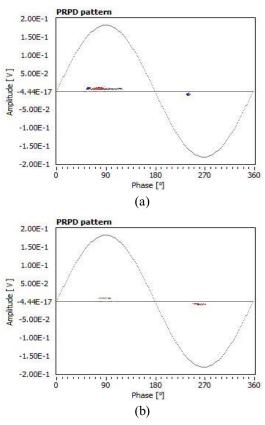
Fig. 4. Partial discharge pattern was obtained for needleplane electrode configuration of (a) SF+0.05wt% SiO<sub>2</sub> (b) SF+0.1wt% SiO<sub>2</sub>. Test voltage 30 kV
