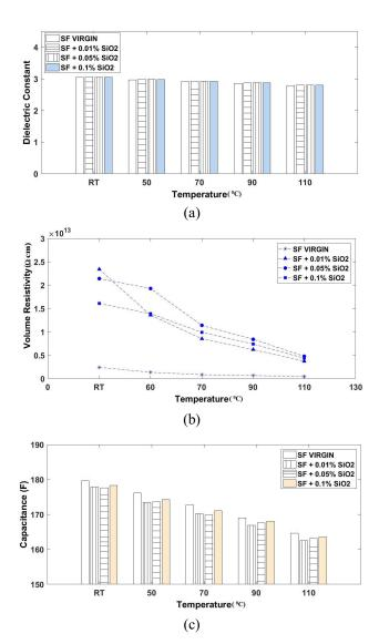
Fig. 10. Comparison of Virgin and nano modified sunflower oil at different temperature (a) Dielectric constant, (b) Volume Resistivity, (c) Capacitance
