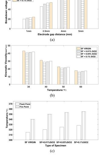
Fig. 8. Comparison of Virgin sunflower oil with nano modified sunflower oil (a) Breakdown Strength, (b) Viscosity, (c) Flash and Fire point
