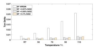
Fig. 9. Tan-Delta test for virgin sunflower oil and nano modified sunflower oil at different temperature
