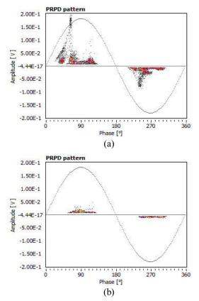
**Fig. 3.** Partial discharge pattern was obtained for needleplane electrode configuration of (a) SF Virgin (b) SF+0.01wt% SiO<sub>2</sub>. Test Voltage 30 kV.
