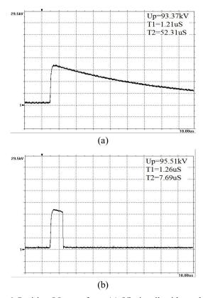
Fig. 6. Positive LI waveform (a) Virgin oil withstand (b) Virgin oil breakdown
