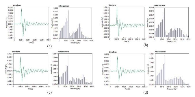
**Fig. 5.** Partial discharge pulses and corresponding frequency spectrum obtained for needle-plane electrode configuration of (a) SF Virgin (b) SF+0.01wt% SiO<sub>2</sub> (c) SF+0.05wt% SiO<sub>2</sub> (d) SF+0.1wt% SiO<sub>2</sub>.Test voltage 30 kV
