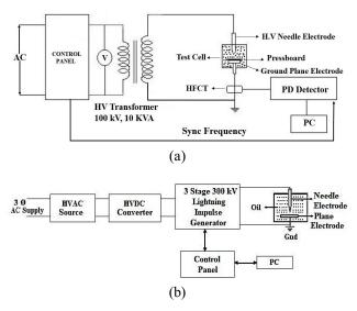
Fig. 1. Schematic diagram of the experimental setup for needle-plane electrode configuration (a) PD test, (b) 300 kV, 3 stage Lightning Impulse
