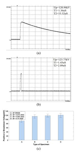
Fig. 7. (a) 0.1wt% SiO<sub>2</sub> nano sample withstand (b) 0.1wt% SiO<sub>2</sub> nano sample breakdown. (c) Comparison of Positive LI breakdown voltage of virgin oil specimen with different nano oil specimen
