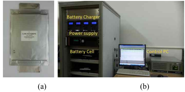
Fig. 7. Experiment condition for single cell test. : (a) Battery cell. (b) Experimental equipment for single cell test
