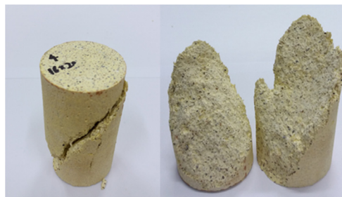
Fig. 4. Failure surface and distribution of grains inside an artificial sedimentary rock. This specimen contains 40% coarse grains
