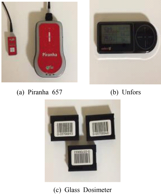
Fig. 2. (a) The Piranha 657, (b) Unfors, (c) Glass dosimeter were used to measure entrance surface dose.
