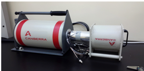
Fig. 1. HPGe detector for measurement of delayed gamma-ray from the ^{nat}W sample.
