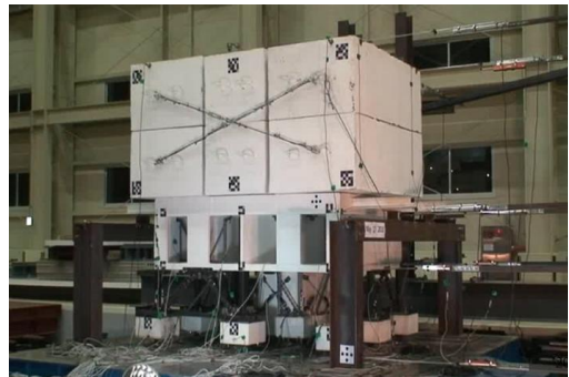
(b) Shake-table test of 1:5-scale model
