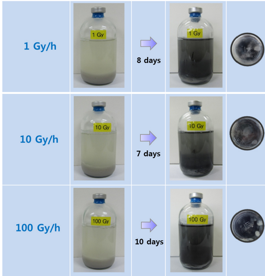
Fig. 5. Color changes of the bentonite samples that were treated with different intensities of \gamma -irradiation have occurred during their anaerobic incubation for several days.
