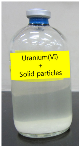
Fig. 1. A serum bottle that contains uranium(VI), solid particles, and hydrogen gas in anaerobic water.
