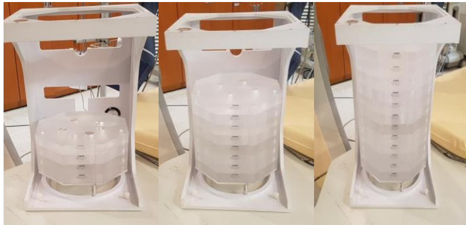
(a) Thin adult (b) Normal adult (c) Heavy adult Fig. 1 NEMA Phantom's diagonal arrangement between tube and detector
