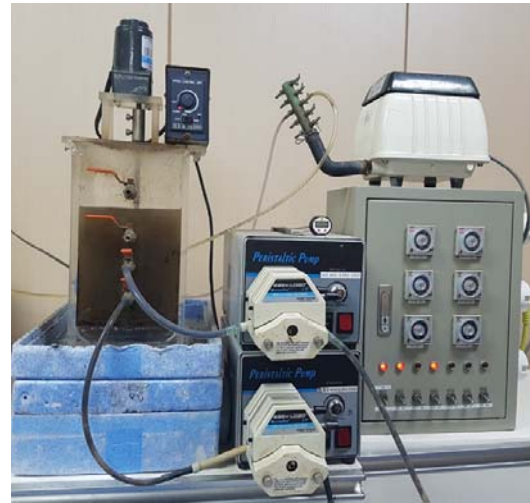
Fig. 1. Lab. scale SBR reactor.
