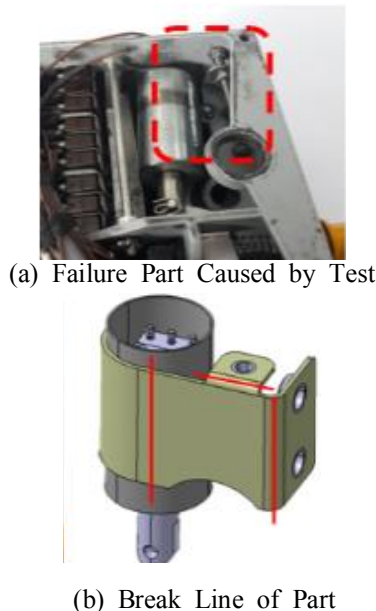
Fig. 5 Failure of Solenoid Bracket by Gunfire Vibration Test
