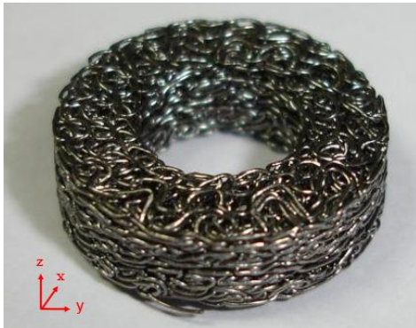
Fig. 3 Configuration of SMA Mesh Washer[8]
