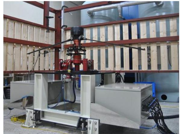
Fig. 5 Small-scaled Tip Jet Test Aparatus
