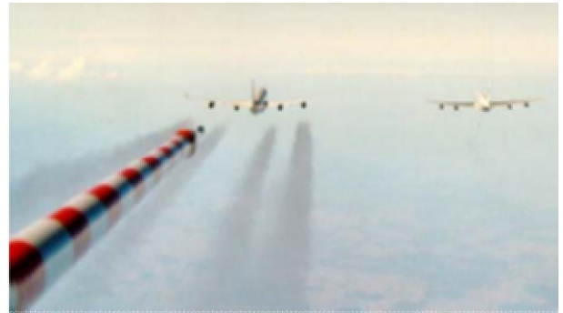
Fig. 4 Left: B707 with relatively low propulsion efficiency. Right: A340 with relatively high propulsion efficiency[6].
