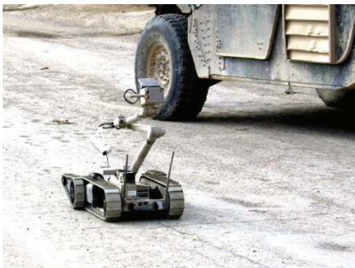
Fig. 1. A robot system for detection and removal of explosive devices.
