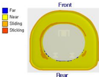
Fig. 19 Contact condition of bottom surface of cap-silicon (case 2)
