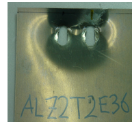
(c) Curling+Tensile crack (ALZ2T2E36)
