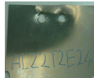
(a) Shear fracture (ALZ2T2E24)
