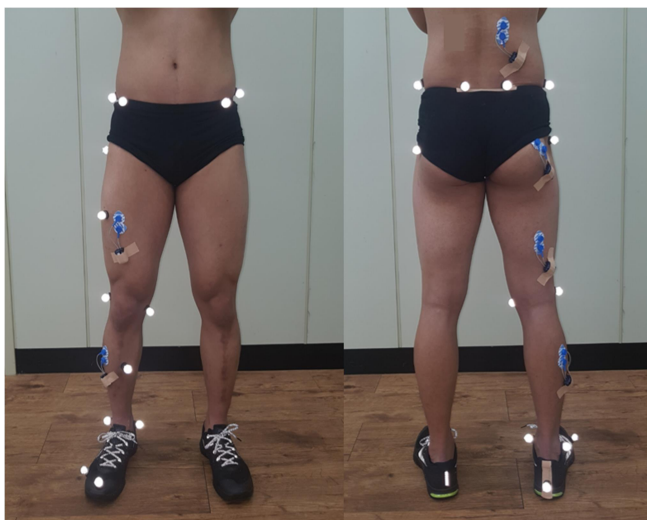
Figure 3. Reflective markers and EMG attachment points.
