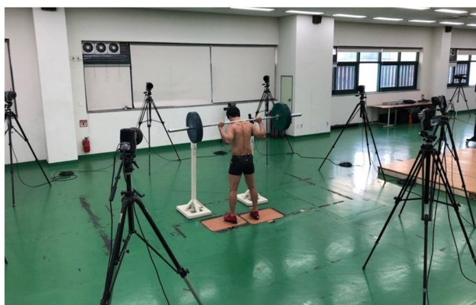
Figure 1. Experimental setup: subject standing on the force plate, facing forward.
