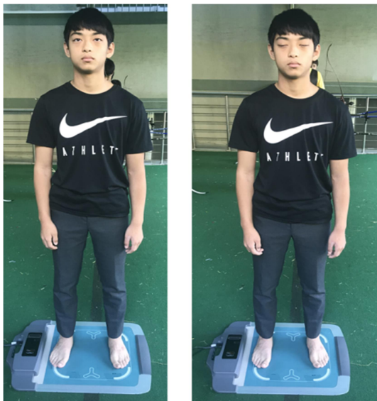
Figure 3. Analysis of static balance of foot plantar pressure with the eyes open and closed
