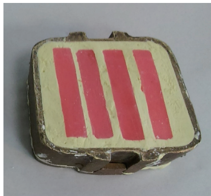
Fig. 1. Arrangement of wax patterns within the flask.
