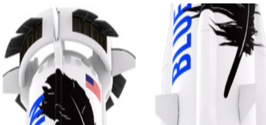
Fig. 12 Control surface of New Shepard[13].
