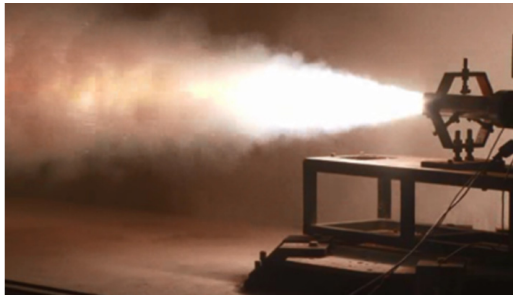
Fig. 3 Ground test for nozzleless booster.
