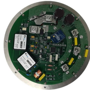
(b) Embedded current controller
