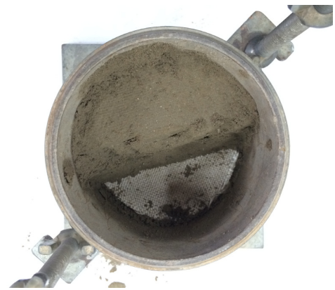
Fig. 3. A Proctor compaction test
