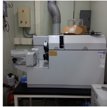
(b) Inductively coupled plasma mass spectrometer (ICP-MS)
