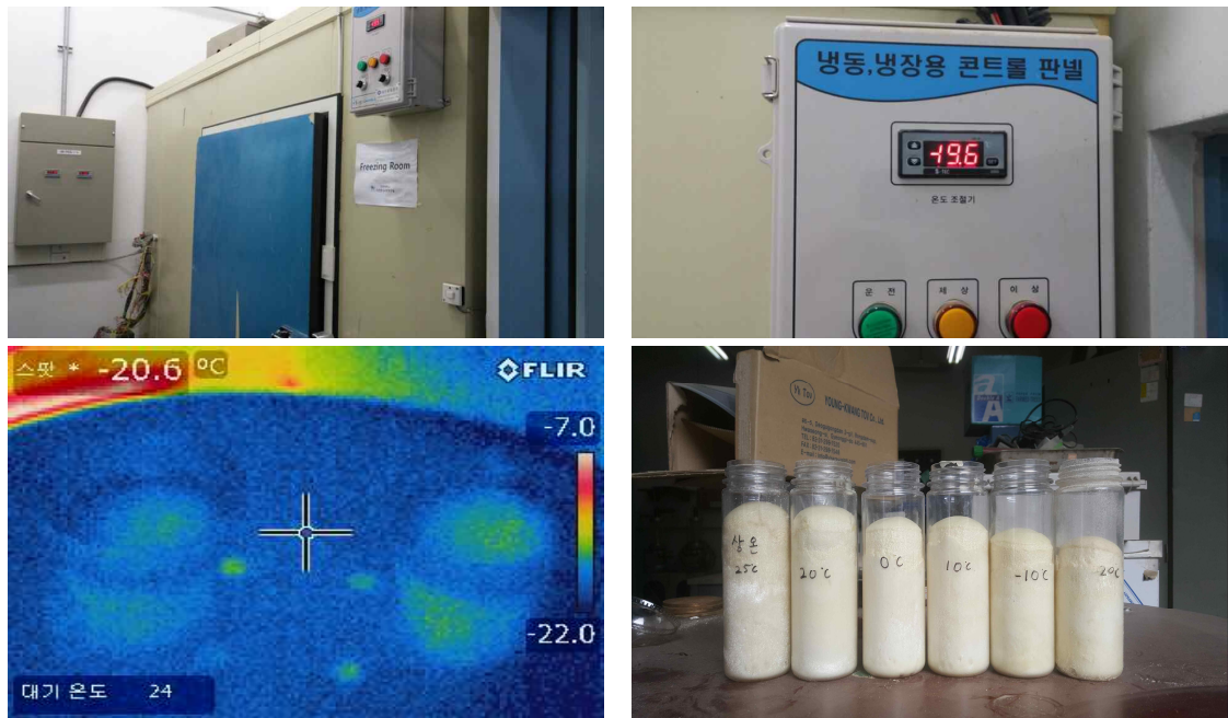
Fig. 4. Temperature chambers and expansion material
