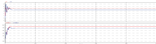
Fig. 8 String current when compensator not used
