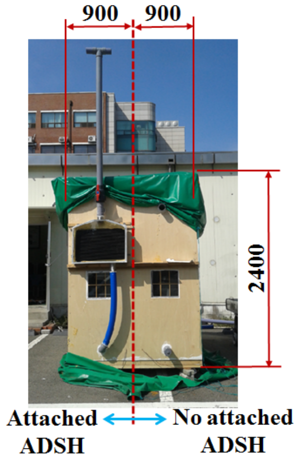
Fig. 4. Experimental house fixed ADSH[8].
