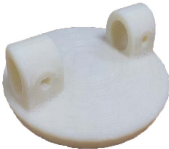
Fig. 11. Optimal butterfly valve disc printed by 3D printer
