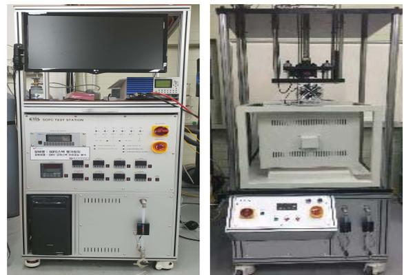
**Fig. 1.** SOFC stack safety performance evaluation system
