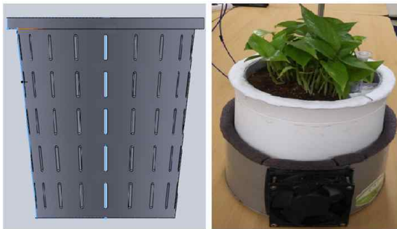
Fig. 2. Inside mesh structure pot and a fan installed near the root zone of the plant.
