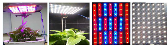
Fig. 1. Mixed light(Red+Blue) and high CRI LED to illuminate the light on plants(A) and LED array structure(B)
