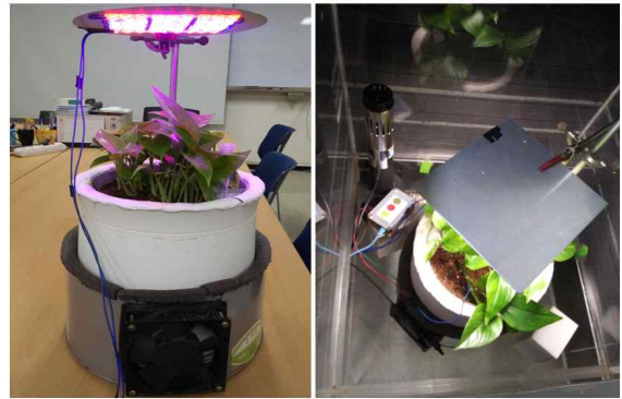
Fig. 3. Indoor Air Purification System equipment(A) and in chamber(B).
