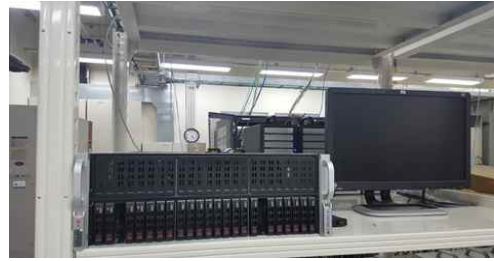
Fig. 4 Implemented SW Digital Filter System using NVIDIA Titan V GPU, Intel XEON CPU, and SAS RAID
