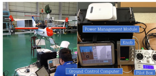
Fig. 8. Configuration of portable ground control system
