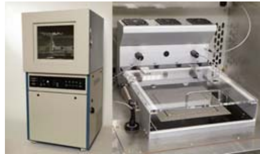
〈Figure 1〉 Sweating guarded hotplate integrated system (SGHO-8.2)
