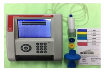
Figure 1. Spirometer, Pony FX MIP/MEP (Cosmed Srl, Rome, Italy).
