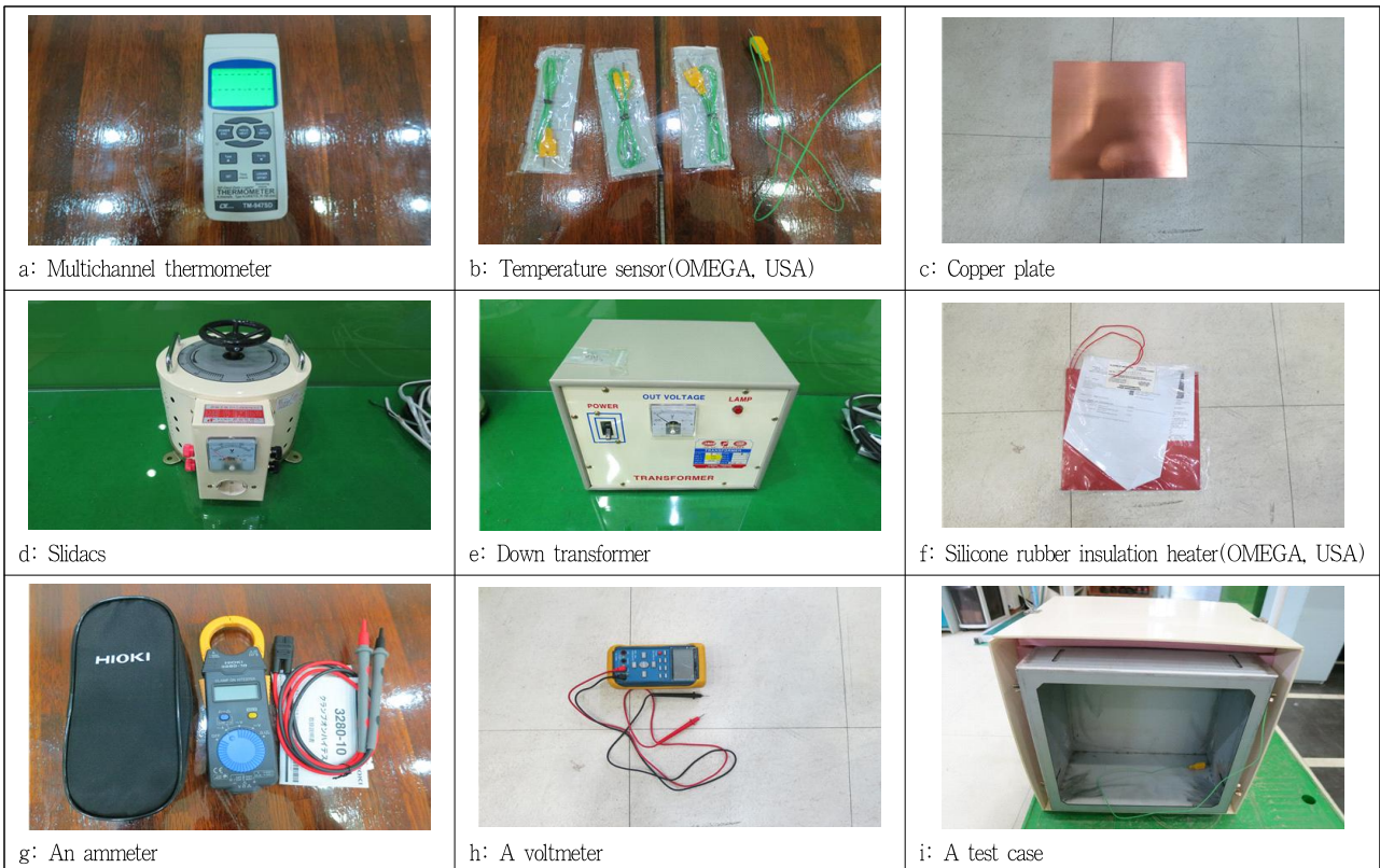
Figure 5. Thermal conductivity (k) measurement equipment
