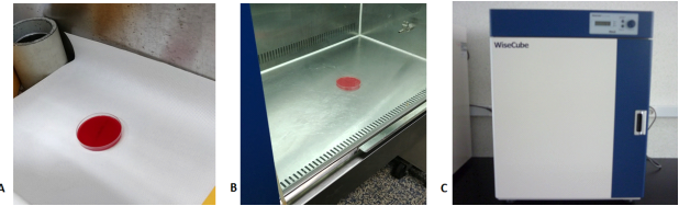
Fig. 3. The left(A) is a collection of falling bacteria from a common workbench, the middle(B) is a collection of falling bacteria from the clean workbench, and the right(C) is an incubator.
